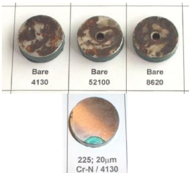
Eliminated Pitting Corrosion For Cr x N Coating on 4130 Steel
