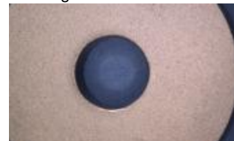
No Wear Debris for X-53 With TiC & a-C Coating vs. Bare X-53
