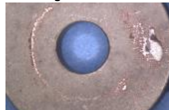
Fretting-Wear Debris for X-53 vs. X-53
